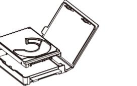
2.Connect SY-ADA20121 with the HDD.
