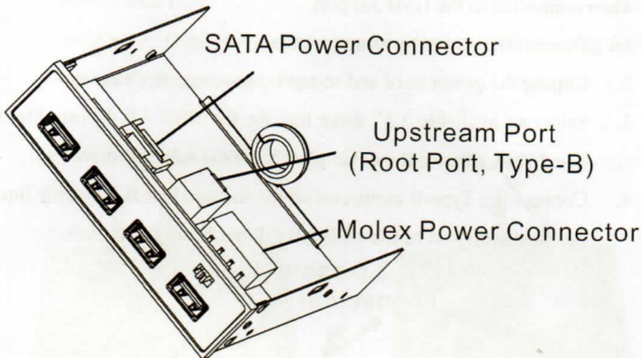
**Figure 1. USB 3.0 4-Port Front Hub Layout**
