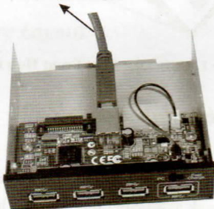
**Figure 2. Connecting the USB 3.0 Cable**
