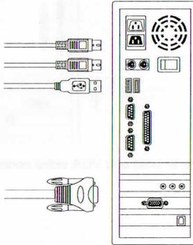
Figure 7: USB & PS/2 (Keyboard & Mouse) and VGA connected
