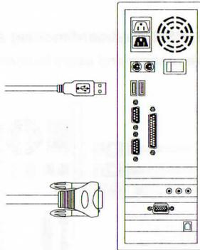
Figure 9: USB and VGA video connected
