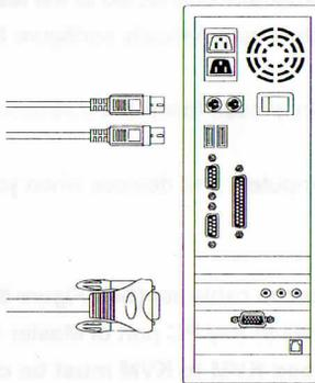
Figure 8: PS/2 (Keyboard & Mouse) and VGA connected
