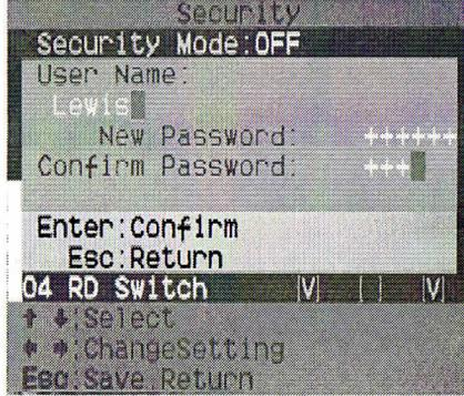
Figure 29: User name password setup window
