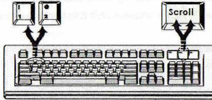
Figure 12: Specific channel selection hot key
