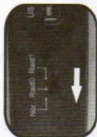
Set the switch on NOR position, press the reset button under power on mode.
