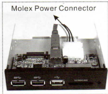
**Figure 3. Connecting the Power Cable**
