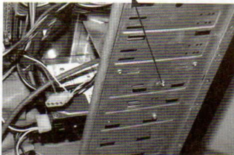
**Figure 4. Mounting the Hub + Card Reader Combo**
