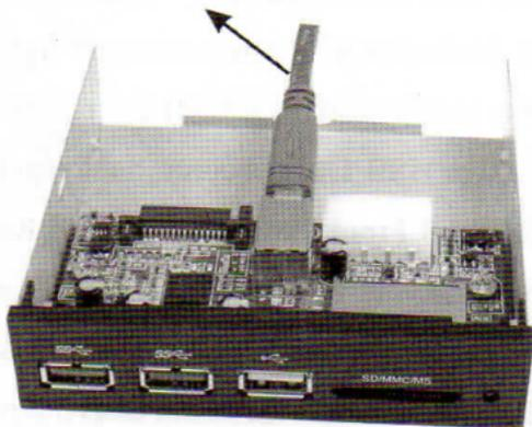
**Figure 2. Connecting the USB 3.0 Cable**
