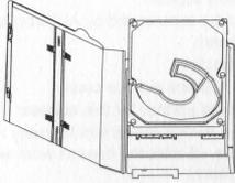
2. Connect SY-ADA20120 with the HDD.
