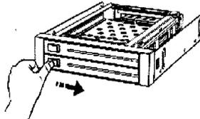
2. Put the 2.5" HDD into the HDD-ROM and close the front panel.
