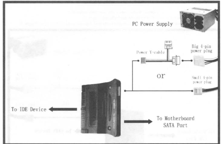
Figure 1: IDE Device to motherboard's SATA Port connection
