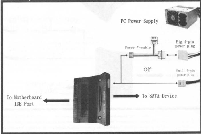
Figure 3: SATA Device to motherboard's IDE Port connection
