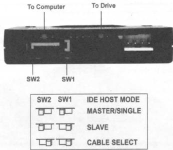
Figure 2: Master/Slave/Cable Select mode configuration
