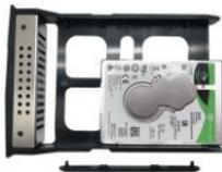
1. Remove the clasp on the right side of the extraction disk, and place the 2.5-inch hard disk in the position shown on the left.
